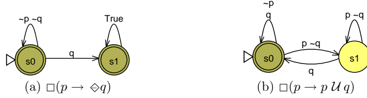
Fig. 1. Two PTL formulae and their respective equivalent Büchi automata. In the state transition diagrams, True is a shorthand representing any input symbol from the alphabet set \{pq, p\sim q, \sim pq, \sim p\sim q\} , \sim p any input symbol from \{\sim pq, \sim p\sim q\} , and q any input symbol from \{pq, \sim pq\} . The double-circled states in darker shade are accepting states.
