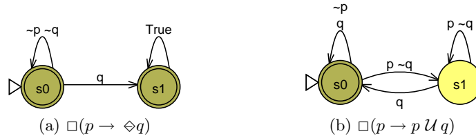
Fig. 1. Two PTL formulae and their respective equivalent Büchi automata, where the double-circled darker states are accepting states. Note that True is a shorthand representing any input symbol from \{pq, p\sim q, \sim pq, \sim p\sim q\} and q representing any input symbol from \{pq, \sim pq\} .
